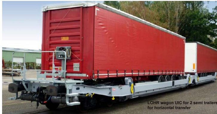
Wagons Lohr UIC Blocs of 9 double platforms linked by draw bars
