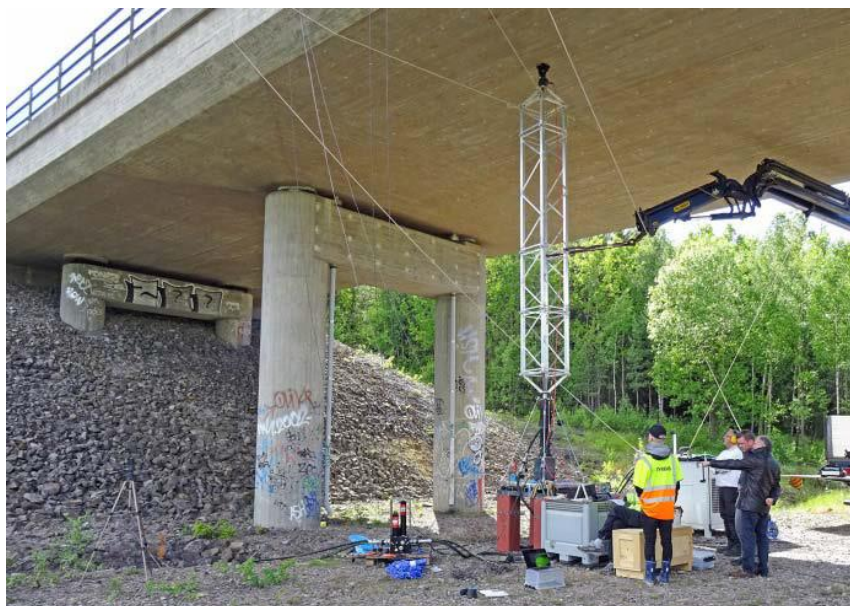
FIGURE 42. THE BEAM BRIDGE AT PERSHAGEN, DURING TESTING WITH THE HYDRAULIC EXCITER
