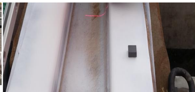
Place marker A at the beginning of the measuring location and marker B at the end of the measuring location
