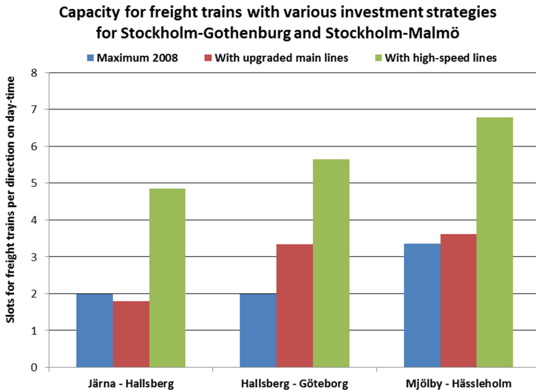
Figure 5.8: Number of possible train slots for freight trains during daytime on different double track sections on the mainlines Stockholm-Gothenburg/Malmö, at 2008 with maximum speed 200 km/h, with upgraded main lines to 250 km/h and with real high-speed lines built.
