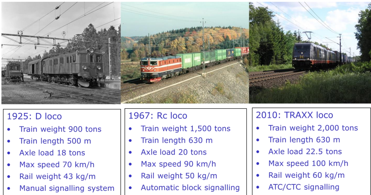
Figure 7.8: Tractive power, freight trains and infrastructure in a historical perspective, example from Sweden.
