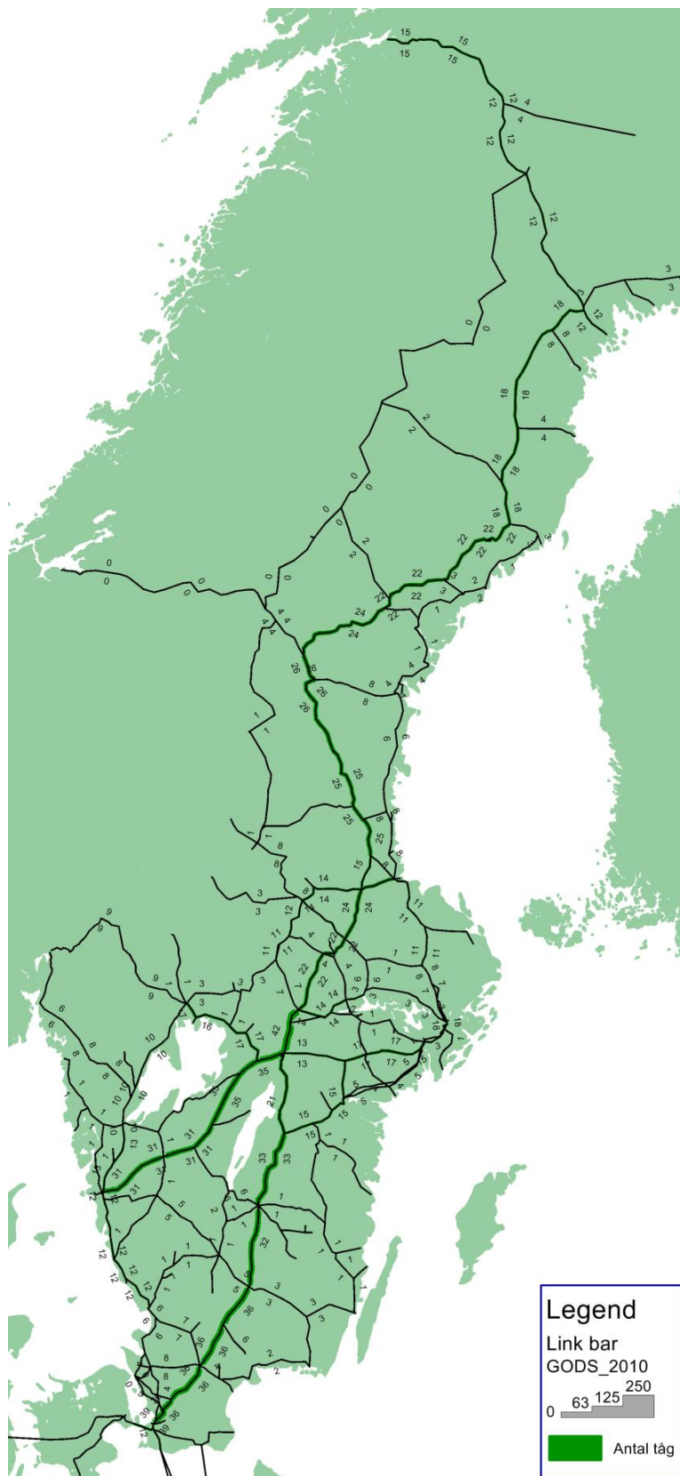
Figure 4.1: Number of freight trains per section and direction on the railway network in Sweden 2010. The figures are planned trains, the actual number of operated trains are lower.
