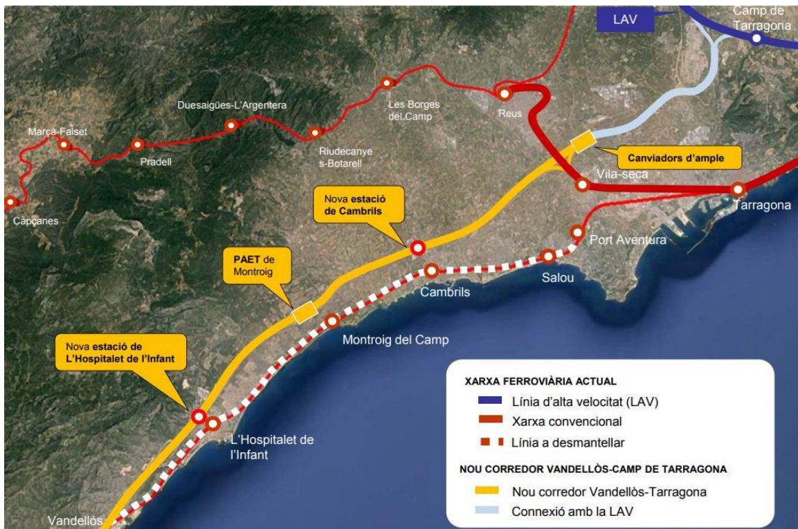
FIGURE 32 SITUATION OF THE SECTION VANDELLÒS – VILASECA (6)
