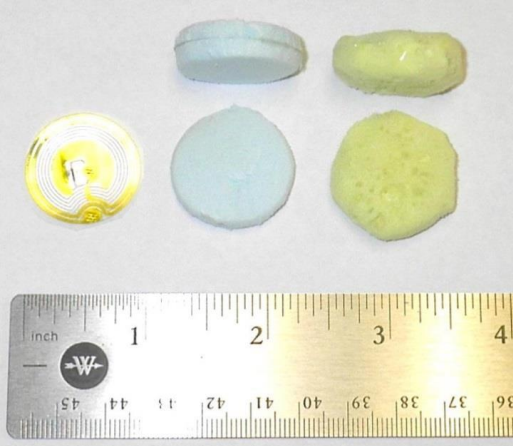
Figure 33. RFID tags encased using extruded polystyrene (centre) and polyurethane spray foam (right ) [15]
