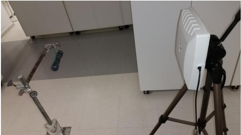
Figure 39. Test for reading distance without obstacles except the PVC coating
