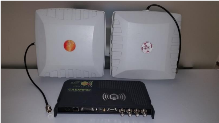
Figure 36 Used equipment (clockwise) in tests: a) Directional antenna; b) Cylindrical antenna; c) RFID Reader
