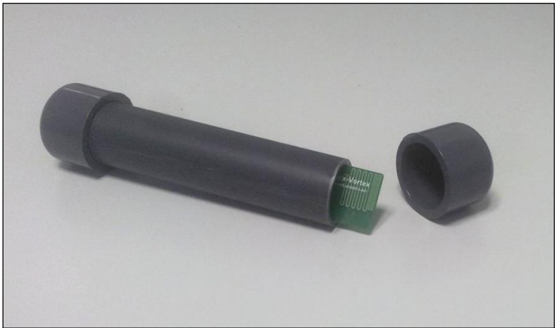
Figure 38. PVC coating with the RFID sensor tag inside
