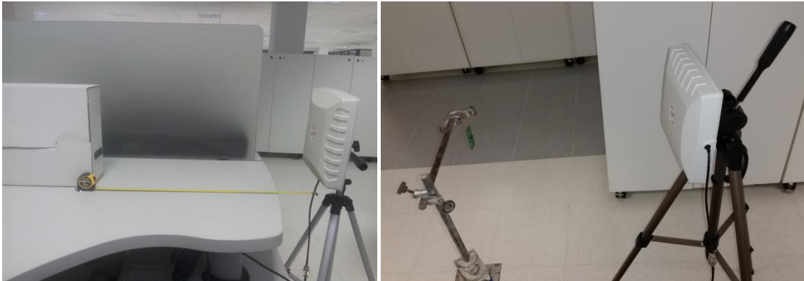
Figure 37. Test for reading distance without obstacles
