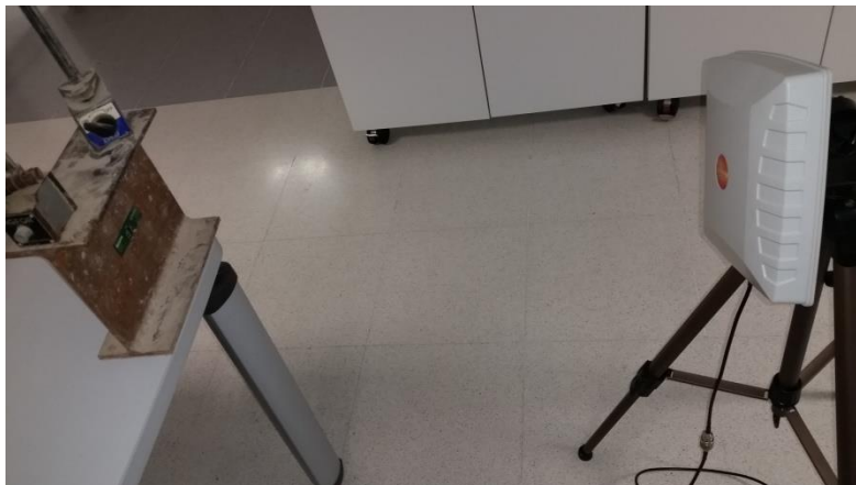
Figure 42 Test for reading distance with the influence of a metal plate
