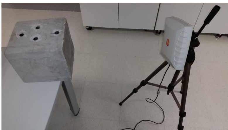
Figure 46 Configuration to test the attenuation of concrete
