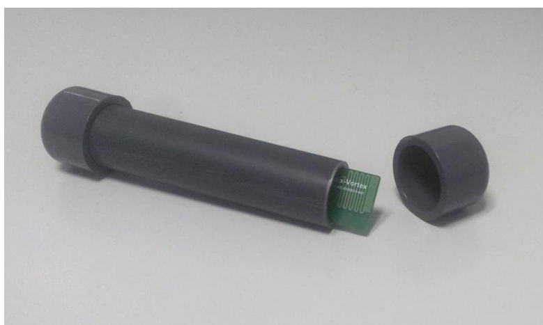
Figure 34. PVC encapsulation selected for RFID sensor tags
