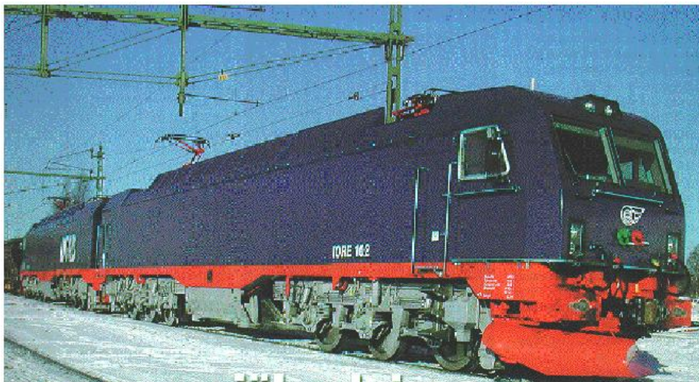
Figure 4.8: IORE electric twin locomotive for iron ore transport in northern Sweden.
