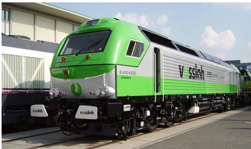
Figure 4.10: Euro 4000 diesel-electric locomotive for freight and passenger transport.
