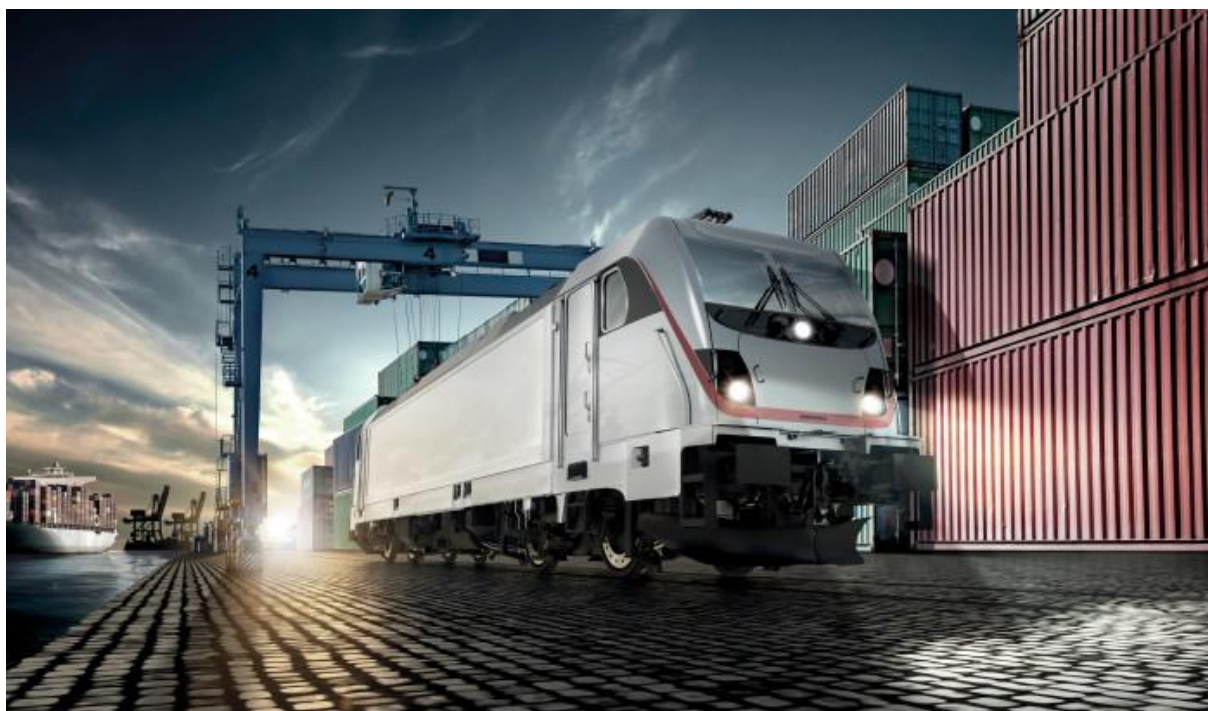
Figure 4.12: Duo-locomotive with both electric and diesel traction, Traxx “Last mile”.
