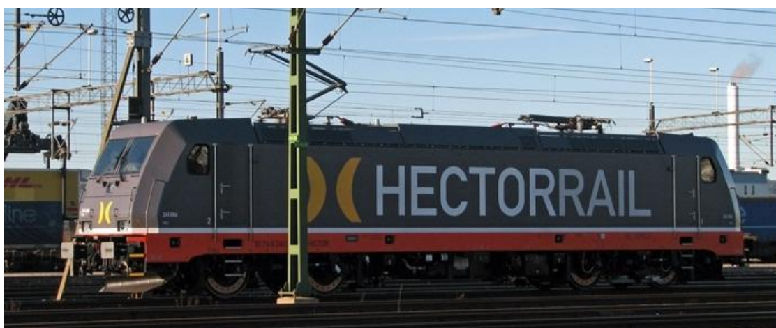
Figure 4.9: TRAXX electric locomotive for freight and passenger transport (example)
