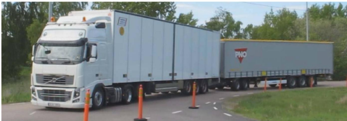
Figure 3:5: In Sweden 32 m long trucks for two 40 ft containers and a possible maximum weight of 90 tonnes are being tested at the same time as an extension of 18 m trucks to 25 metres is being discussed within the EU.
