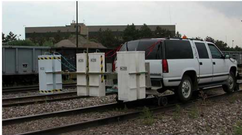
Figure4.1.9 – GPR rail-setup with three pairs of 1-GHz horn antennas (Selig et al., 2003).
