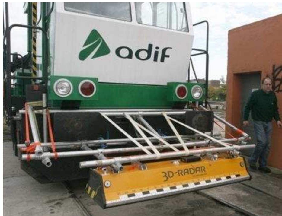
Figure 4.1.12. 3D-Radar GPR system tested mounted on the front of an ADIF maintenance train.
