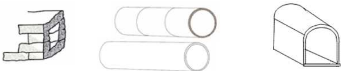
Figure 4.2.29. Different types of culverts, Södergren (2011)
