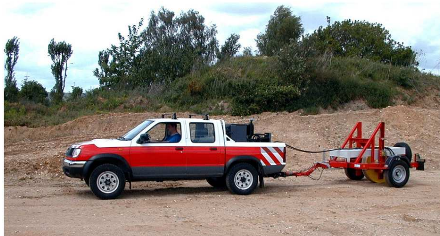
Figure 4.1.6 – The “Portancemetre” apparatus (INNOTRACK, 2010).
