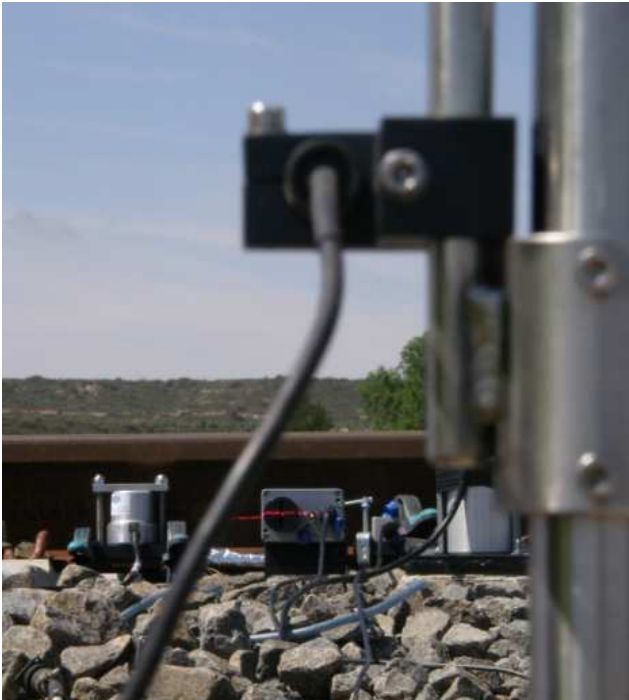
Figure 4.1.7 – Laser system used for measuring rail deflections directly
