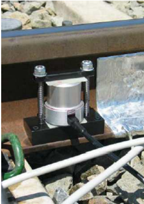
Figure 4.1.8 – Geophone of 2 Hz provided with the adequate support to be clamped to the base of a standard rail
