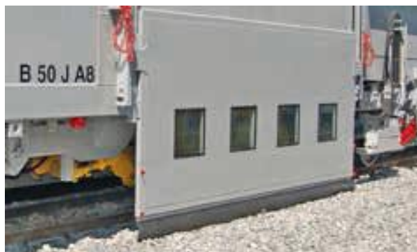
Figure 21. Soundproof panels to reduce tamping noise. Matisa [30]
