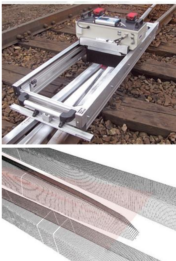
Figure 3.2.59. Graw Scorpion S&C measurement system (source http://graw.com )
