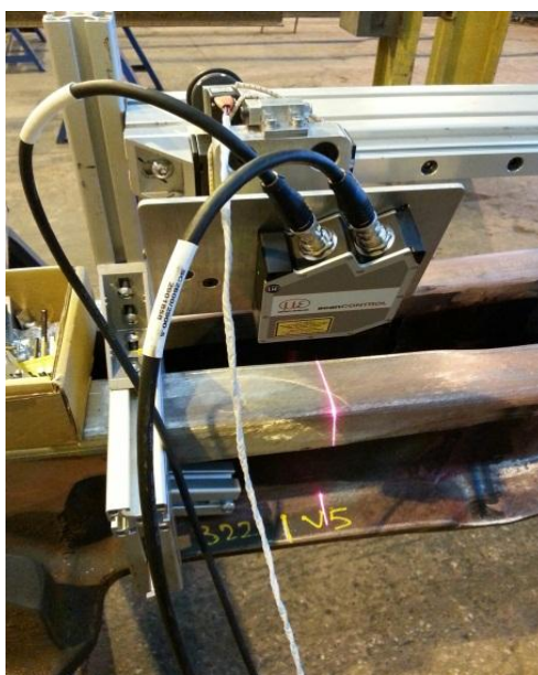
Figure 3.2.58. UoH Laser measurement on welded leg end
