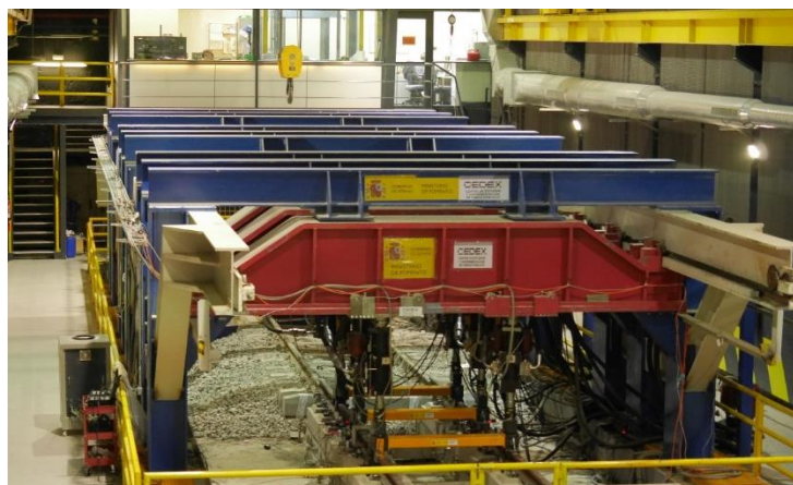
FIGURE 6 – CAPACITY4RAIL DEMONSTRATOR CARRIED OUT IN THE CEDEX TRACK BOX
