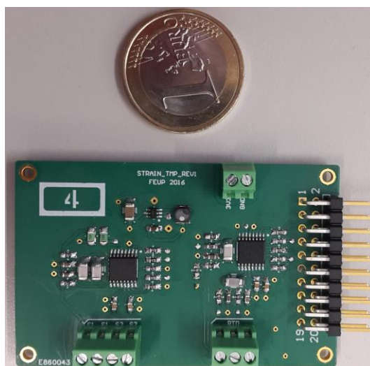
FIGURE 12 - STRAIN AND TEMPERATURE MODULE - FIRST PROTOTYPE
