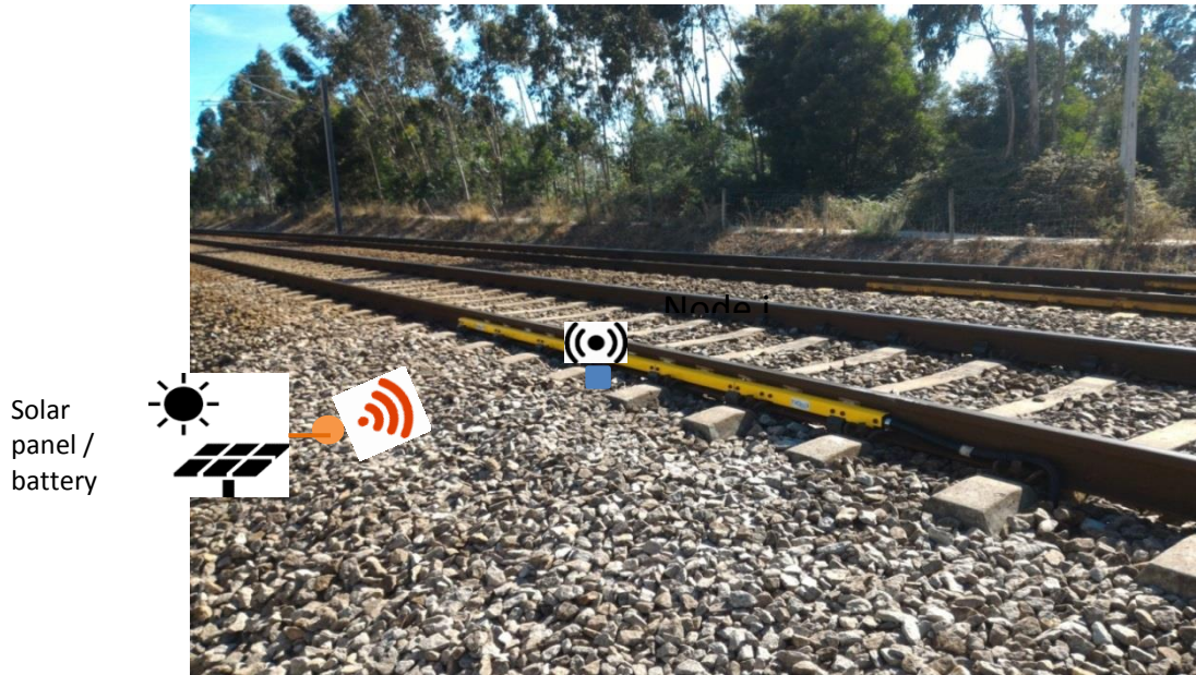
FIGURE 31 – WEIGHING IN MOTION AND WHEEL DEFECT DETECTION
