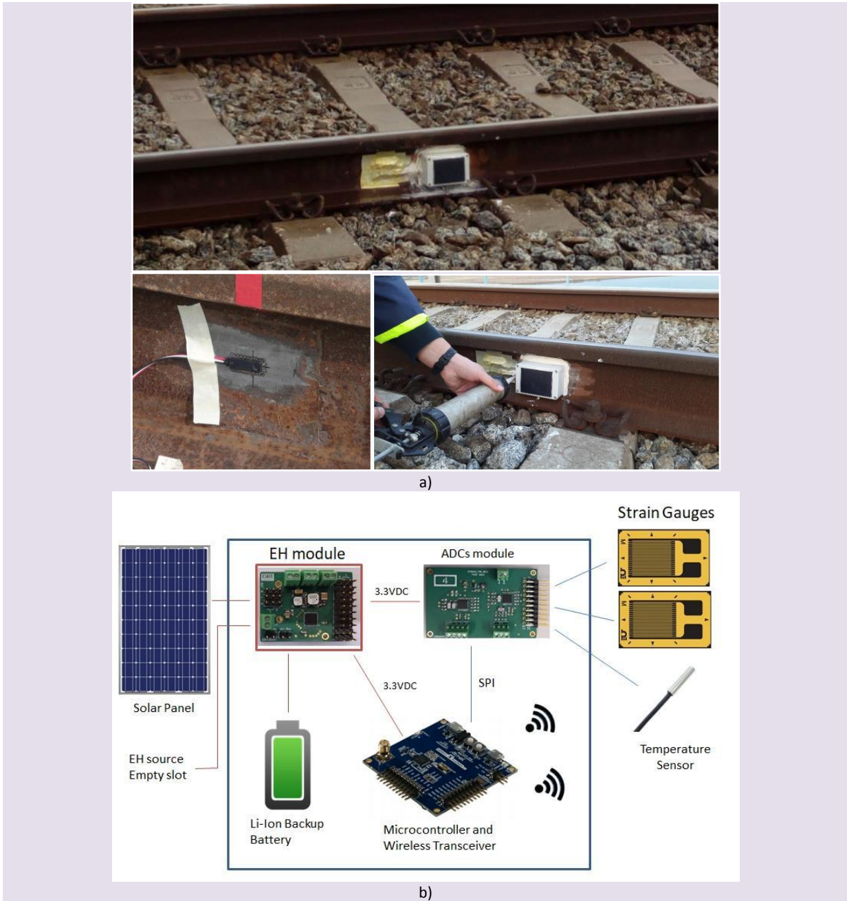
FIGURE 18 – SENSOR NODE 1 INSTALLATION A) AND SCHEME B)
