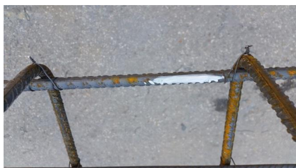
FIGURE 6. POLISHING THE SURFACE OF THE BARS OF THE SLAB TRACK PROTOTYPE
