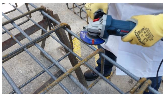
FIGURE 6. POLISHING THE SURFACE OF THE BARS OF THE SLAB TRACK PROTOTYPE
