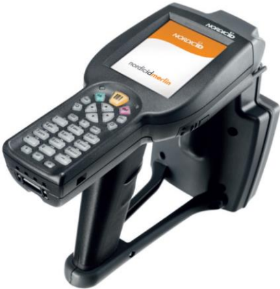
FIGURE 18. HANDHELD RFID READER (NORDIC ID MERLIN UHF RFID CROSS DIPOLE ONE)
