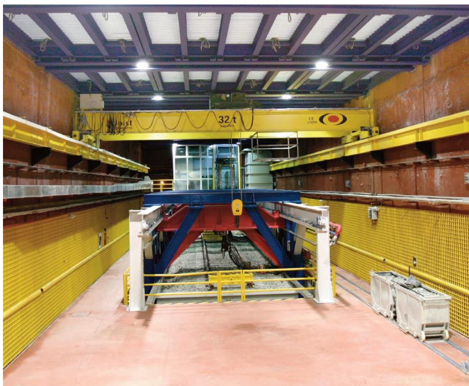
FIGURE 16. GENERAL VIEW OF CEDEX TRACK BOX
