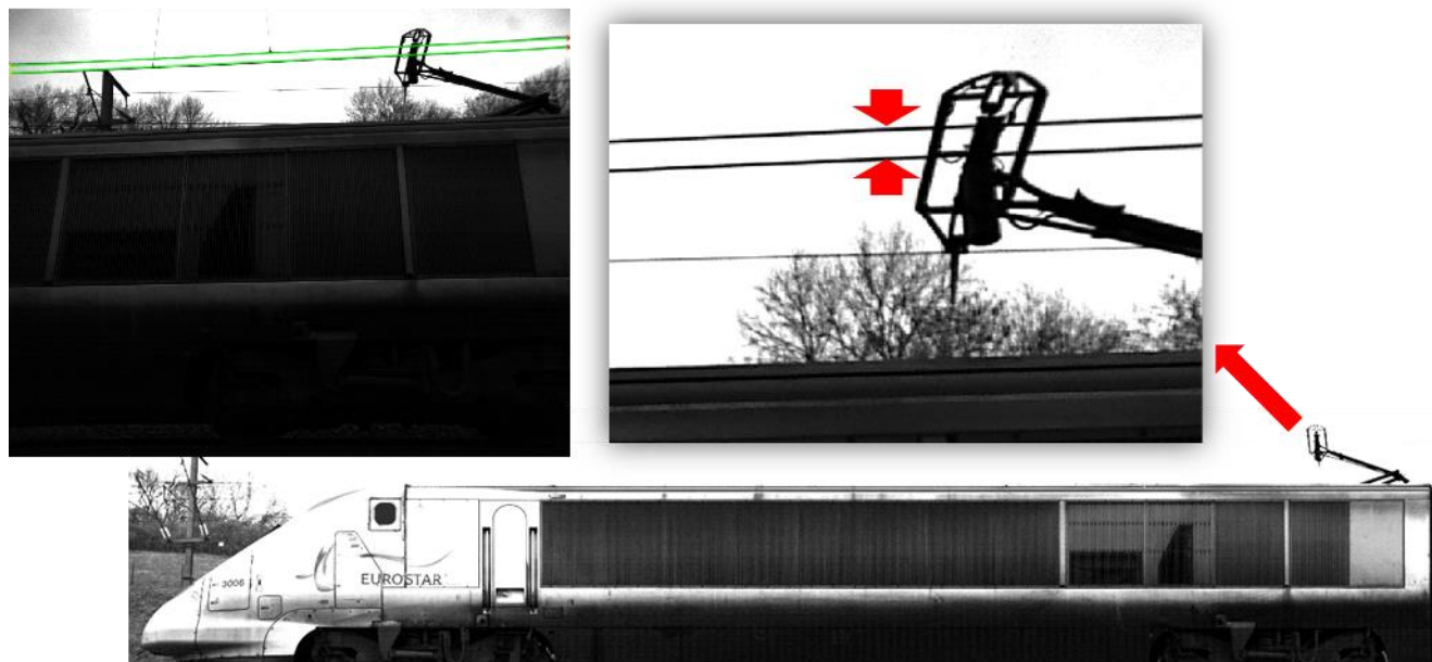
FIGURE 9: MONITORING THE OVERHEAD LINES MOVEMENTS USING FASTCAM UX100
