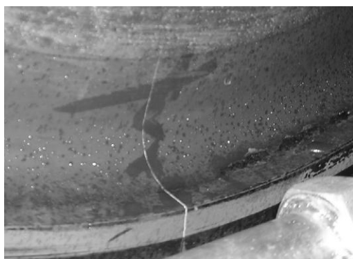
Figure 9 Thermal fracture of a railway wheel extending into the wheel disc 29 .
