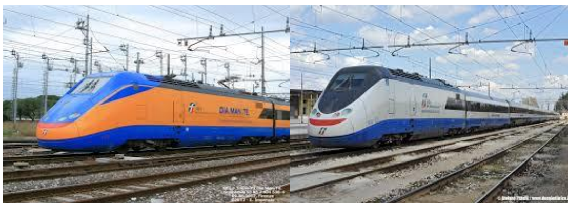
Figure 24 Italian diagnostic trains: DIAMANTE (on the left) and ARCHIMEDE (on the right)
