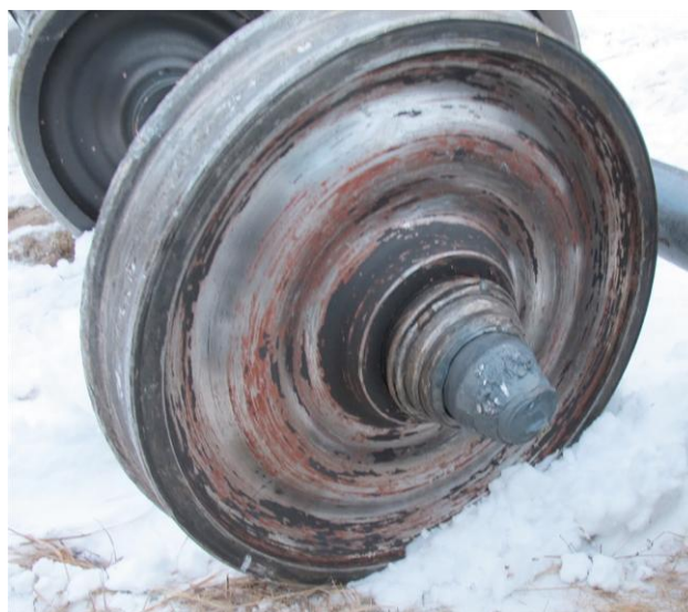
Figure 10 Thermal fracture of a wheelset axle 31
