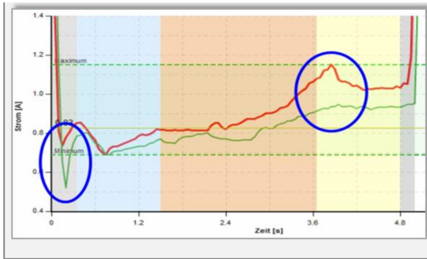
FIGURE 7 TRADITIONAL SWITCH/POINT MONITORING; MEASUREMENT OF THE CURRENT AS A FUNCTION OF TIME
