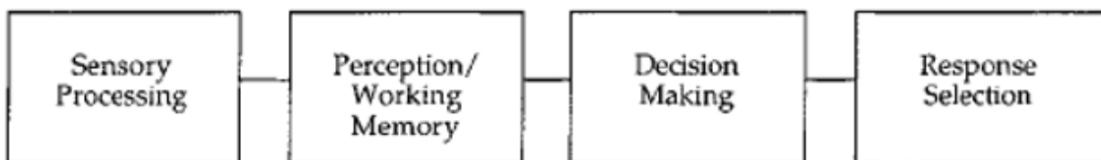
FIGURE 4-4-1 FOUR-STAGE MODEL OF HUMAN INFORMATION PROCESSING (PARASURAMAN, SHERIDAN, & WICKENS, A MODEL FOR TYPES AND LEVELS OF HUMAN INTERACTION WITH AUTOMATIONS, 2000).
