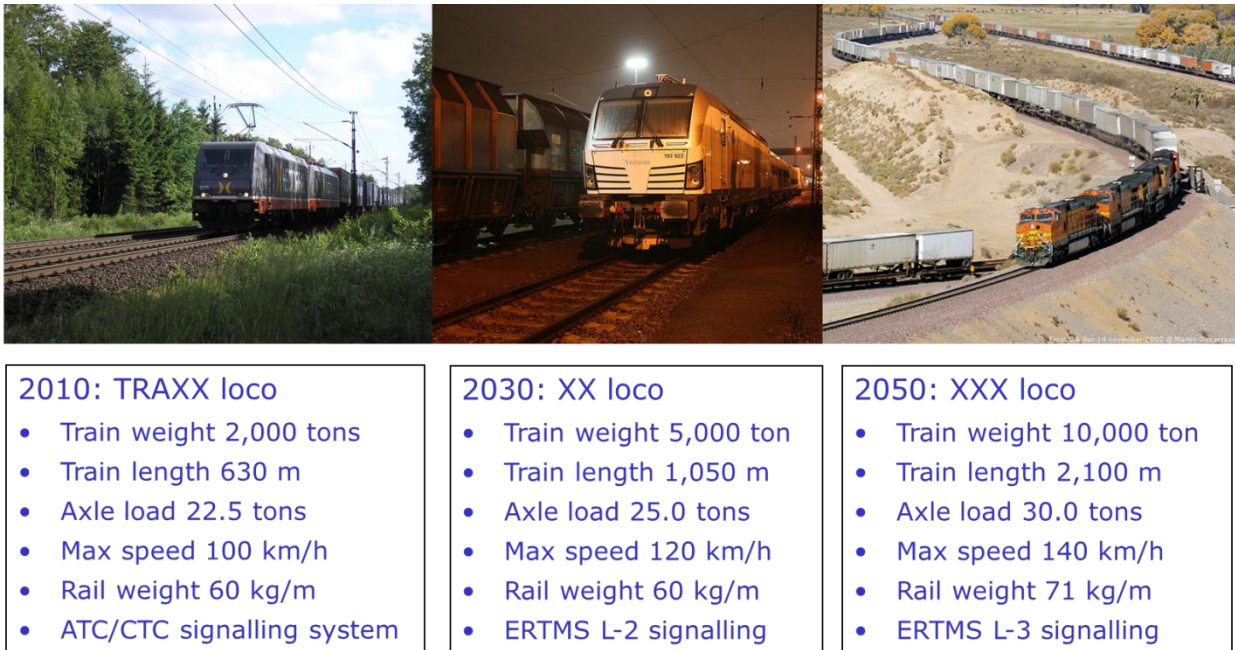
Figure 5.1.3: Tractive power, freight trains and infrastructure in a future perspective.
