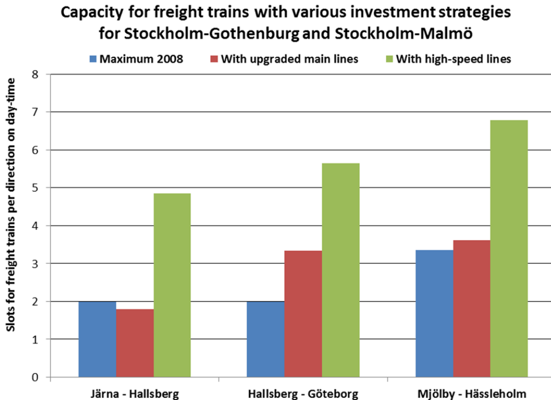
Figure 3.4.4: Number of possible train slots for freight trains during daytime on different double track
