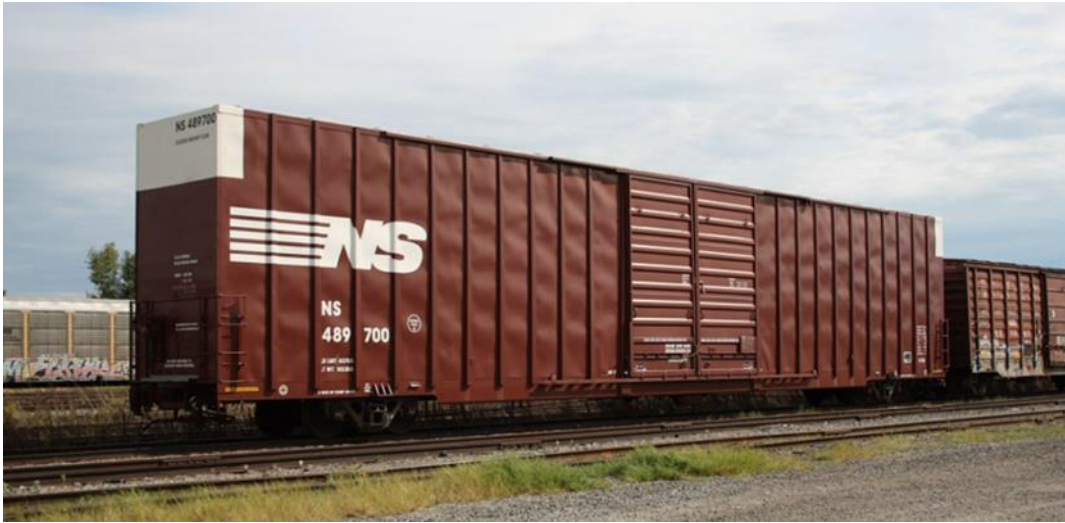
Figure 4.2.10: 4-axle US bogie-wagon Jumbo box car with a loading capacity of 323 m 3 .
