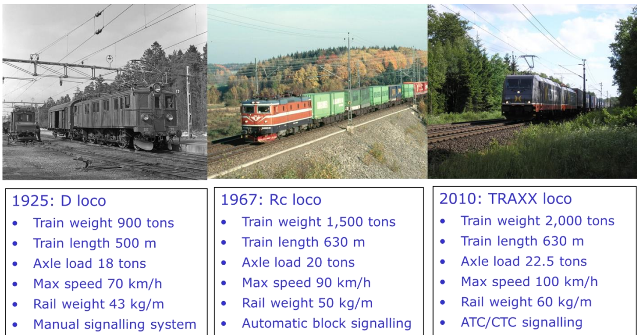
Figure 5.1.2: Tractive power, freight trains and infrastructure in a historical perspective, example from Sweden.
