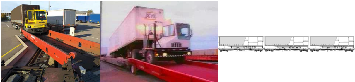
FIGURE 5 MOST OF THE TRAILERS ARE NOT LIFTABLE, THEREFORE ROLL-ON OFF/ROLL ON TECHNIQUE IS AN ALTERNATIVE. LEFT: THE MODALOHR SYSTEM WITH SPECIAL RAMP ON EACH WAGON. MIDDLE: TRAILER TRAINS ONLY NEED A RAMP AT THE END OF THE TRAIN BUT A LOW WAGON AND A HIGH LOADING GAUGE. RIGH A TRAILER TRAIN ARE MORE SPACE EFFICIENT THAN A TRAIN WITH A POCKET WAGON. SOURCE KTH IN CAPACITY4RAIL DELIVERABLE D23.2.
