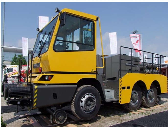
FIGURE 4 COMBINED ROAD-RAIL TRACTOR.
