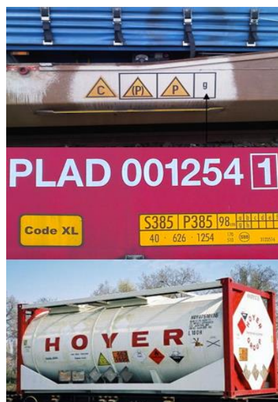
FIGURE 15 DATA LABELS ON A TYPICAL MULTIMODAL TRANSPORT UNIT
