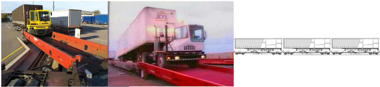
Figure 5.7: Most of the trailers are not liftable, therefore roll-on off/roll on technique is an alternative. Left: The Modalor system with special ramps on each wagon. Middle: Trailer Trains only need a ramp at the end of the train but a low wagon and a high loading gauge. Right: A Trailer Train are more space efficient than a train with pocket wagons. Source: KTH.
