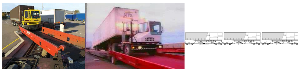
FIGURE 3: A) MODALOHR SYSTEM WITH SPECIAL RAMPS ON EACH WAGON. B) TRAILER TRAINS ONLY NEEDING A RAMP AT THE END BUT LOW WAGONS AND A HIGH LOADING GAUGE. C) TRAILER TRAIN MORE SPACE EFFICIENT THAN TRAIN WITH POCKET WAGONS.
