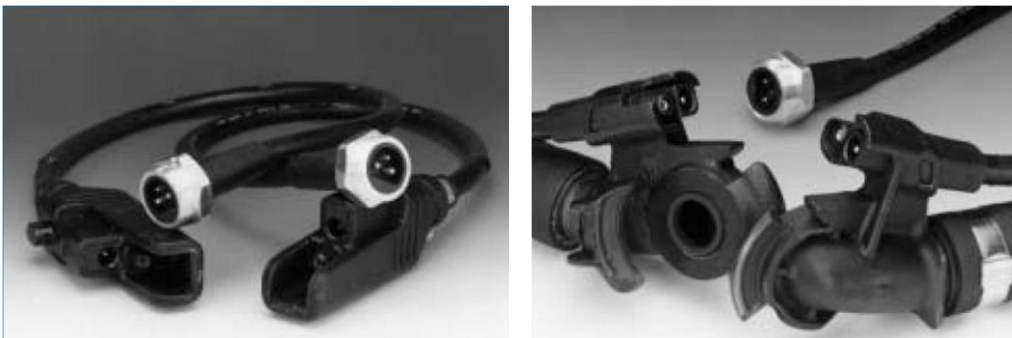
Figure 30: Inter-car-cable with connector and variant sitting on hose couplings (Amphenol). – Source: KB
