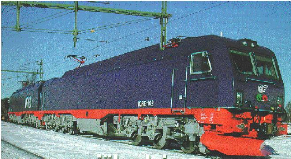
Figure 4.9: IORE electric twin locomotive for iron ore transport in northern Sweden.
