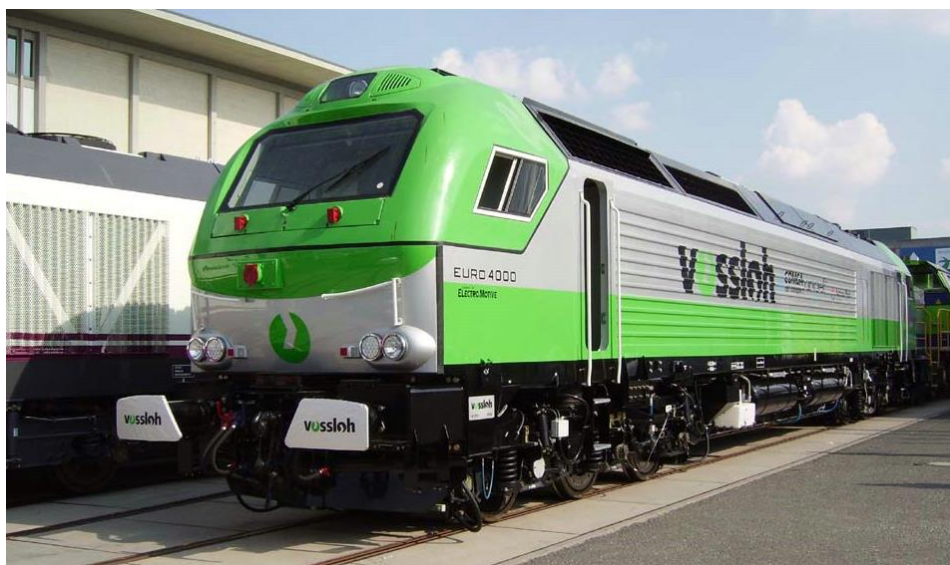
Figure 4.11: Euro 4000 diesel-electric locomotive for freight and passenger transport.
