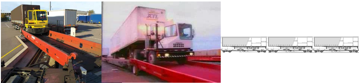
Figure 4.24: Left: Modalohr system with special ramps on each wagon. Middle: Trailer Trains only needing a ramp at the end but low wagons and a high loading gauge. Right: Trailer Train more space efficient than train with pocket wagons.
