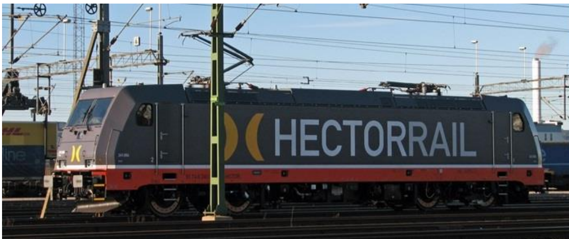
Figure 4.10: TRAXX electric locomotive for freight and passenger transport (example)
