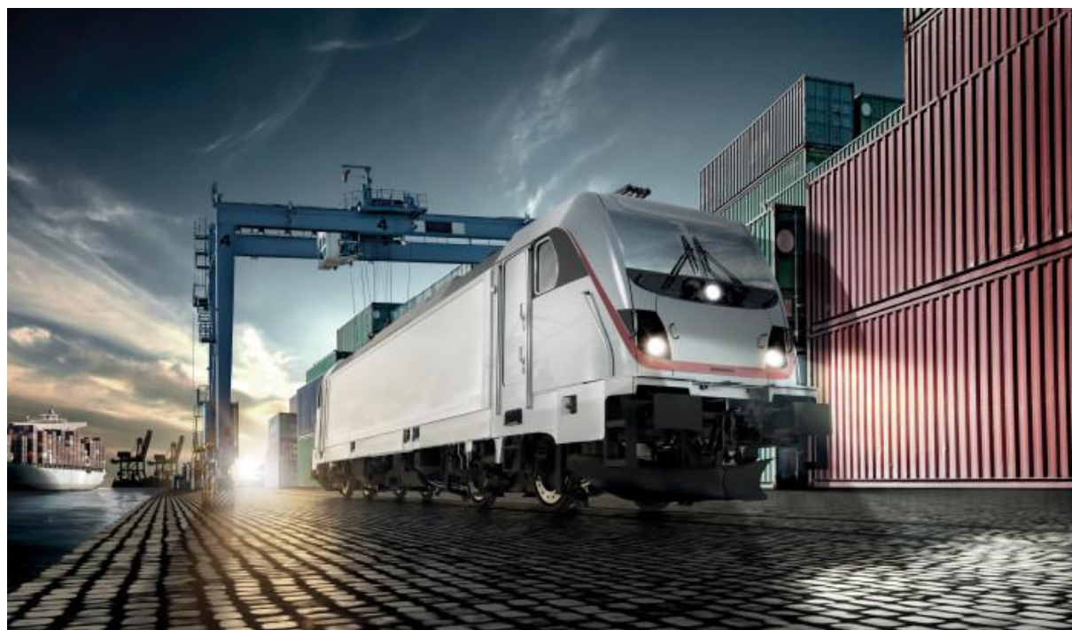
Figure 4.13: Duo-locomotive with both electric and diesel traction, Traxx “Last mile”.
