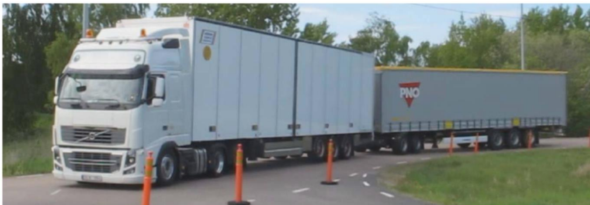
Figure 3:6: In Sweden 32 m long trucks for two 40 ft containers and a possible maximum weight of 90 tonnes are being tested at the same time as an extension of 18 m trucks to 25.25 metres is being discussed within the EU.
