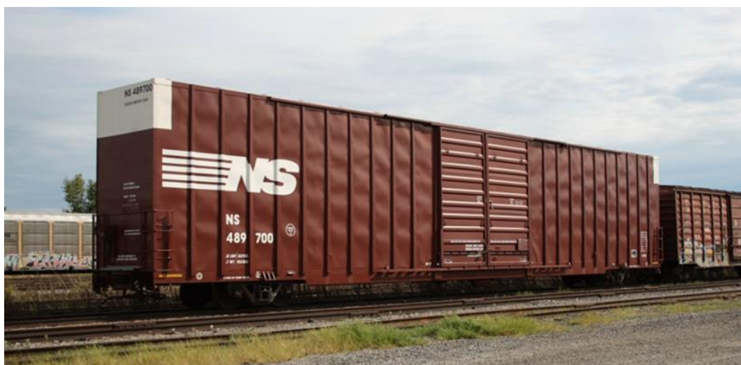
Figure 4.6: 4-axle US bogie-wagon Jumbo box car with a loading capacity of 323 m 3 .
