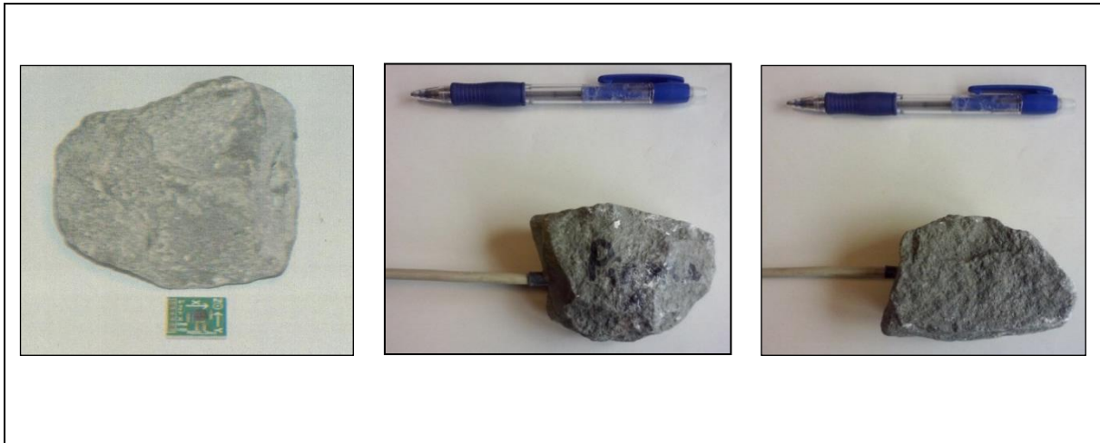
FIGURE 205: PHOTOGRAPHS OF THE TRIAXIAL ACCELEROMETER BEFORE (LEFT) AND AFTER (MIDDLE AND RIGHT) BEING INSTALLED INSIDE THE BALLAST PARTICLE. THE FLAT SURFACE OF THE STONE CAN BE SEEN THE RIGHT PHOTOGRAPH.
