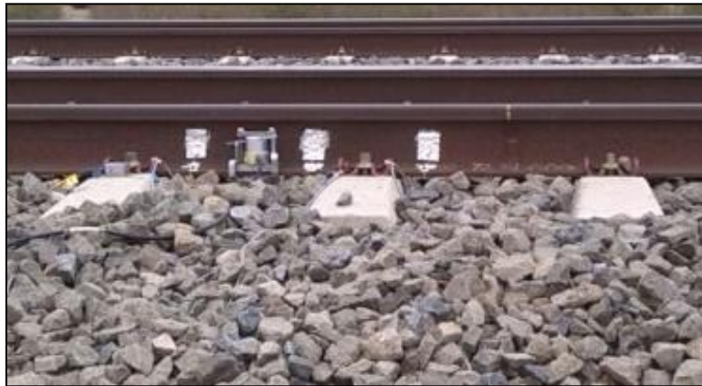
FIGURE 202: PHOTOGRAPH OF THE INSTRUMENTATION IN T-16 AND T-17: SOME STRAIN GAUGES AND A GEOPHONE IN THE RAIL AND ONE ACCELEROMETER, IN THE LEFT SLEEPER
