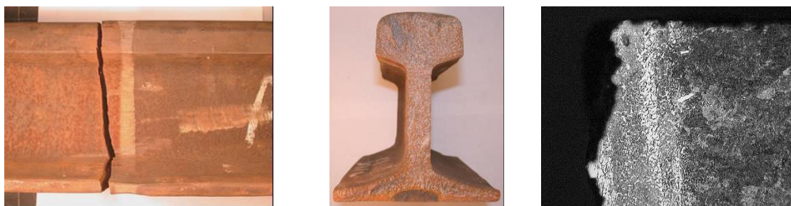
Figure 3.2.57 Example of Fracture from Stainless Insert Interface [3.2.58]
