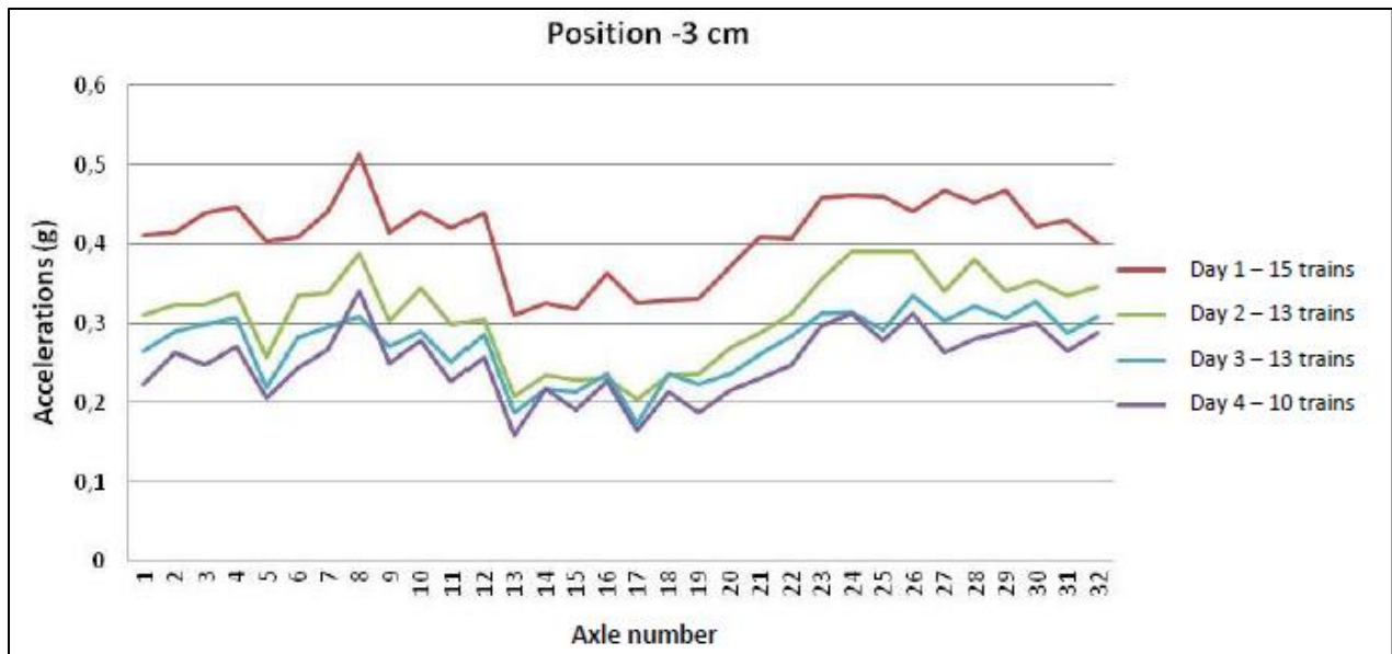
FIGURE 52: BALLAST PARTICLE ACCELERATION AS A FUNCTION OF THE DAYS PASSED SINCE THE PARTICLE PLACEMENT
