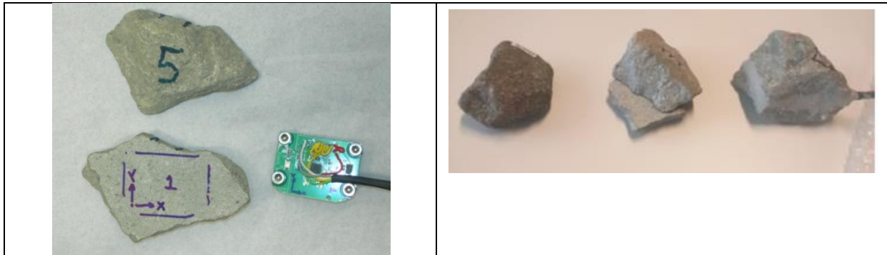
FIGURE 30: BALLAST PARTICLES INSTRUMENTED WITH ACCELEROMETERS
