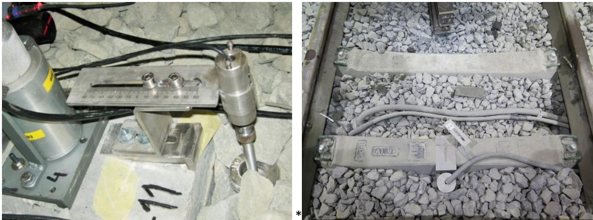
FIGURE 40: LVDT SENSOR HEAD ATTACHED TO ONE SLEEPER
