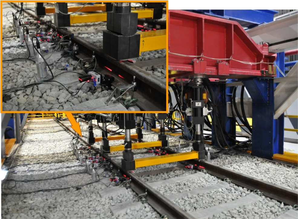
FIGURE 4 VIEW OF THE SURFACE INSTRUMENTATION INSTALLED IN ONE TEST
