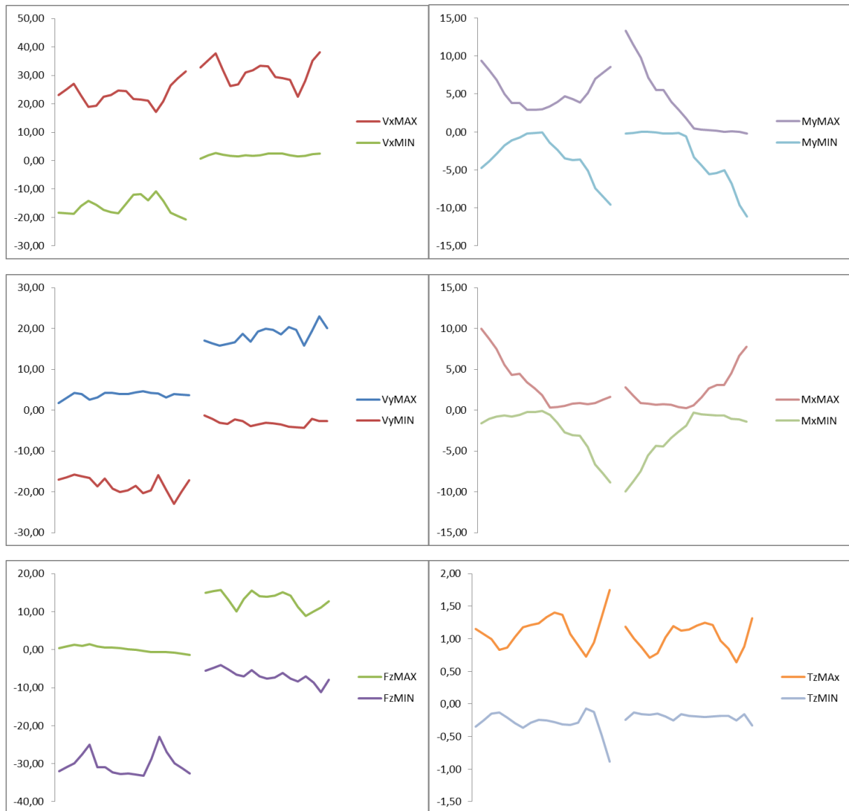
FIGURE 24 : SECTION FORCES ENVELOPES FOR TRANSVERSAL BEAMS
