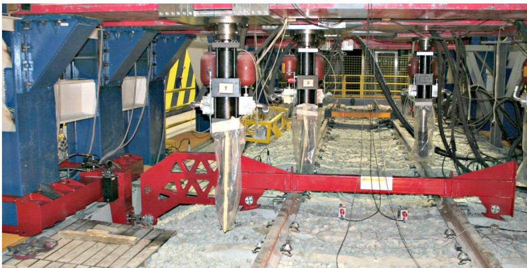
Figure 8: Tool to perform lateral resistance tests mounted on a sleeper
